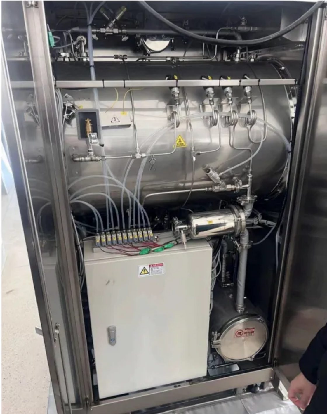
Electropolished chamber and piping surfaces
