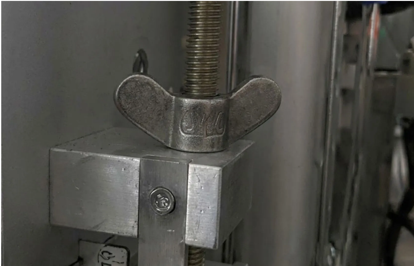
Adjustment supports hollow board thicknesses from 2 mm to 12 mm
