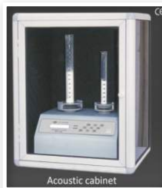
This reduce the sound level to 71 dB to meet laboratory standards
